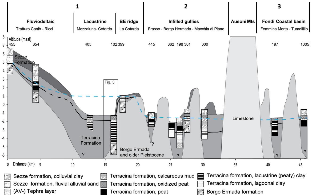
Fig. 2. Cross-section through the Agro Pontino and Fondi basin (based on Van Gorp & Sevink 2019), indicating approximate Early Bronze Age water level of lake and wetland areas (blue line). Names are mentioned once per litho-stratigraphical unit. The legend indicates the lithologies of the core profiles depicted. 1 = inland lake; 2 = south-eastern lake; 3 = Fondi basin; BE = Borgo Hermada; Mts = mountains; AV = Avellino.
