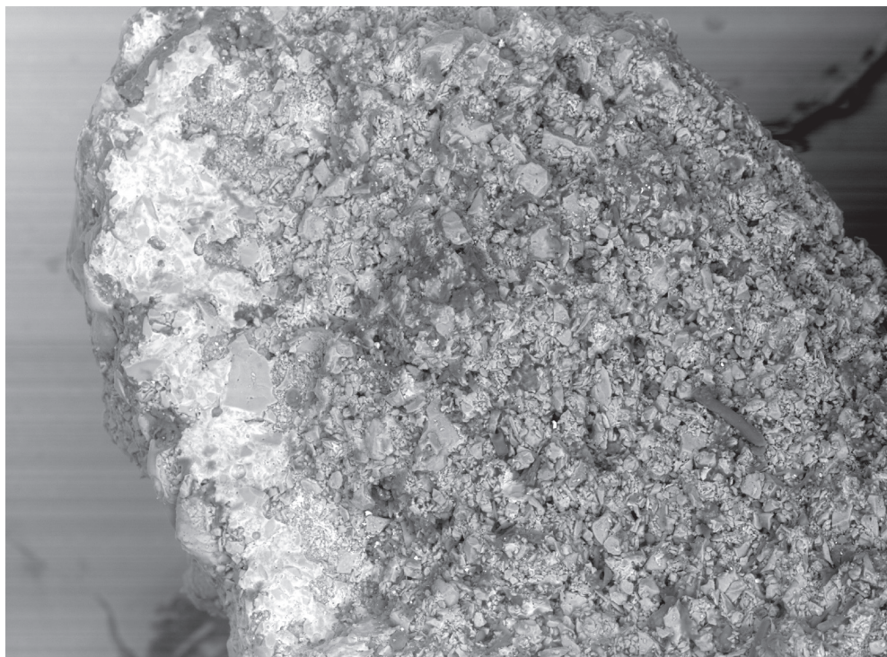
Fig. 12. SEM photomicrograph of the Den Haag-Bronovo faience bead showing the grainy appearance of the bead's fracture surface. The lighter area to the left is glaze on the bead's outer surface (image NMS).
