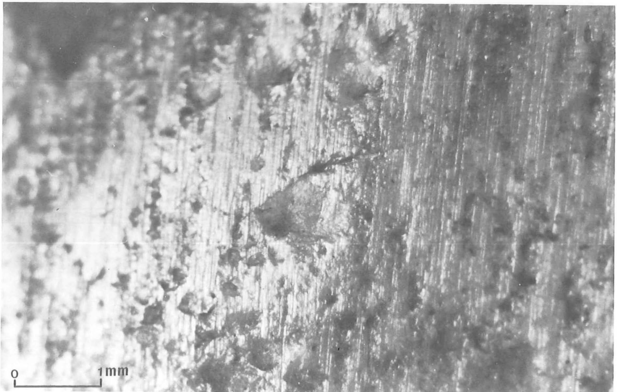
Fig. 13. Grinding scratches on one of the faces of an axe from Ravenswoud (FM 1968-1-8, see fig. 12). The scratches are very regular and strictly parallel, indicating that they were produced with the help of an electrically driven grinding machine. Photo taken by means of a stereomicroscope by D. Stapert.
