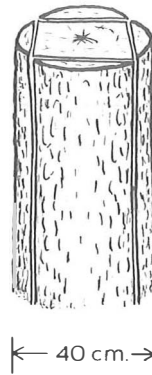
Fig. 24. Slab-wood or slabs, as they are produced by making a square post out of a tree-trunk.
