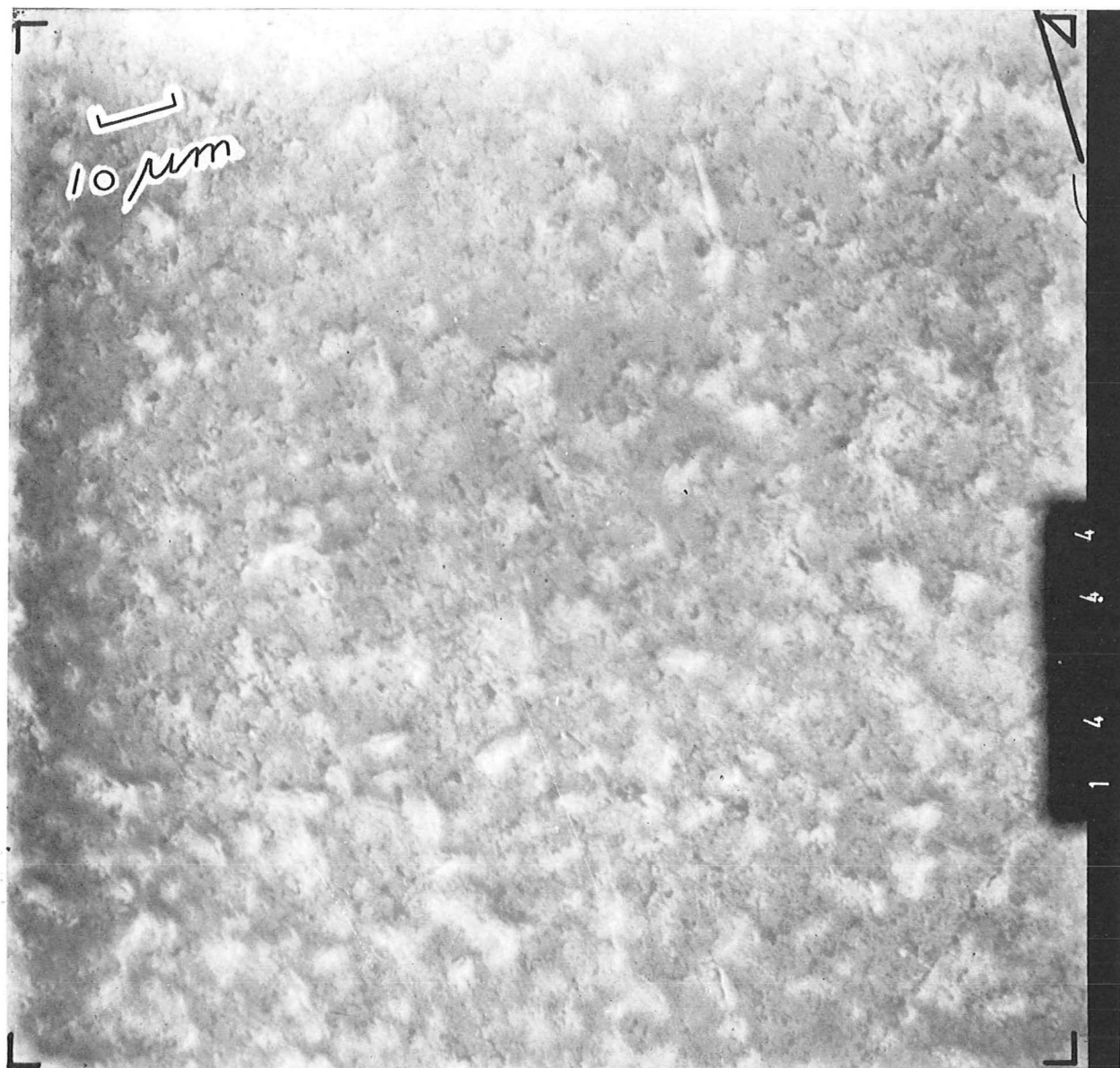
Fig. 8. S.E.M.-photograph of the surface of a (natural) flint from the boulder-sand of Drente, with wind-gloss. The flattening of higher parts of the surface is clearly visible. Photograph by Dr. G. Boom, Laboratory of Physical Metallurgy, Groningen.
