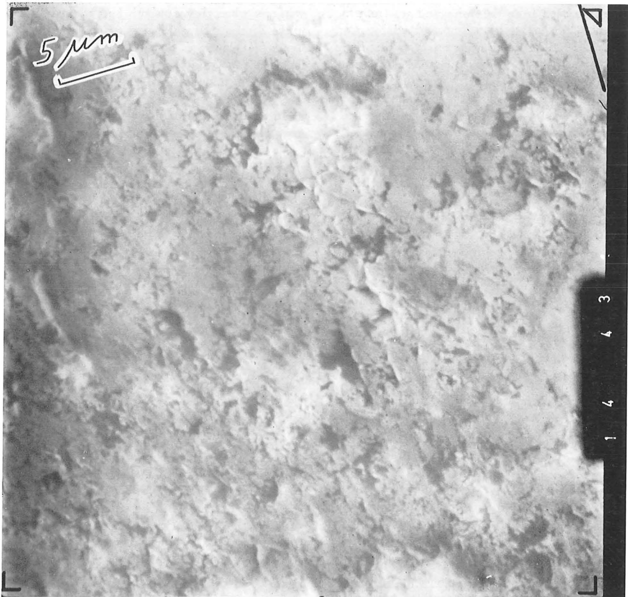
Fig. 9. S.E.M.-photograph of the same surface as in Figure 8, but a higher magnification. The flattened higher parts are clearly visible. The intervening lower areas appear to be unchanged (the normal "plate structure" of flint is visible). Scratches are not present. Photograph by Dr. G. Boom, Laboratory of Physical Metallurgy, Groningen.
